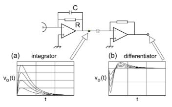
**figure 5** a) Capacitor C integrates the output from the pmt producing an output v(max) of ~Q/C. The reader can verify that a 1 MeV  $\gamma$  producing 6000 photoelectrons will generate a 1 volt output for C = 100 pF with pmt gain = 10<sup>5</sup>.
