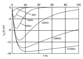
**figure 3** Evaluation of equation (2) for C = 10pF t = 5ns and g =  $10^6$  for various values of R. The amplitude and the shape of the pulses can be easily confirmed with a fast oscilloscope
