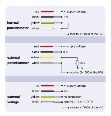
As supplied, the internal potentiometer is set to zero and should be rotated clockwise to increase the voltage when using this control option. When using an external potentiometer to control the HV, the internal potentiometer should be set to maximum (fully clockwise) to provide the correct 2V reference output on the yellow wire. The HV can be monitored by connecting a voltmeter between the white (control) and black (0 V) wires. The HV will be 1000 X the voltage on the white wire.
