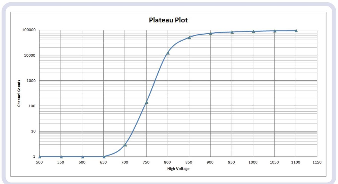
figure 2 signal plateau plot for photomultiplier type 9107B
