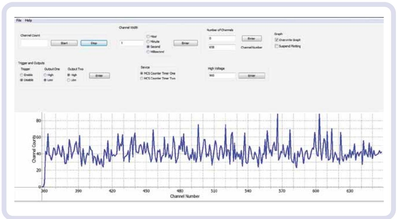
figure 1 dark count run for photomultiplier type 9107B
