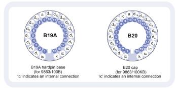
Our range of B19A sockets is available to suit the B19A hardpin base. Our range of B20 sockets is available to suit the B20 cap. Both socket ranges includes versions with or without a mounting flange, and versions with contacts for mounting directly onto printed circuit boards.
