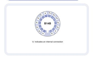
Our range of B14B sockets is available to suit the B14B hardpin base. The socket range includes versions with or without a mounting flange, and versions with contacts for mounting directly onto printed circuit boards.
