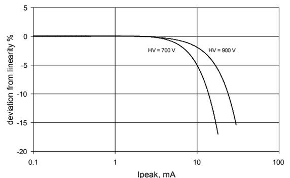
**figure 5** linearity performance for pulses of width  $1 \mu\text{s}$ . The deviation from linear amplification is a limitation of the pmt, and not to the divider.
