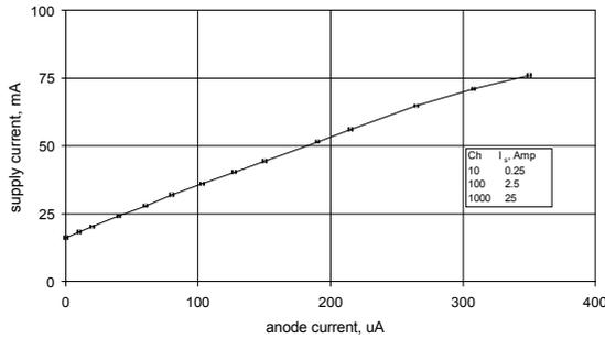
**figure 6** current per channel as a function of mean anode current with 12 V supply. The inset illustrates the low power consumption for multiple channels.
