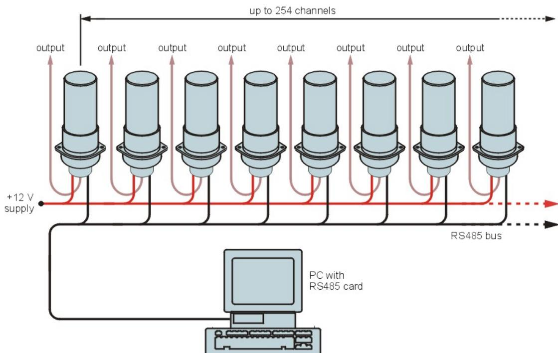
**figure 1** illustrating the system configuration for the control and supply of up to 254 pmts. Only a single 12V supply is required with the HV generated by the individual power bases.
