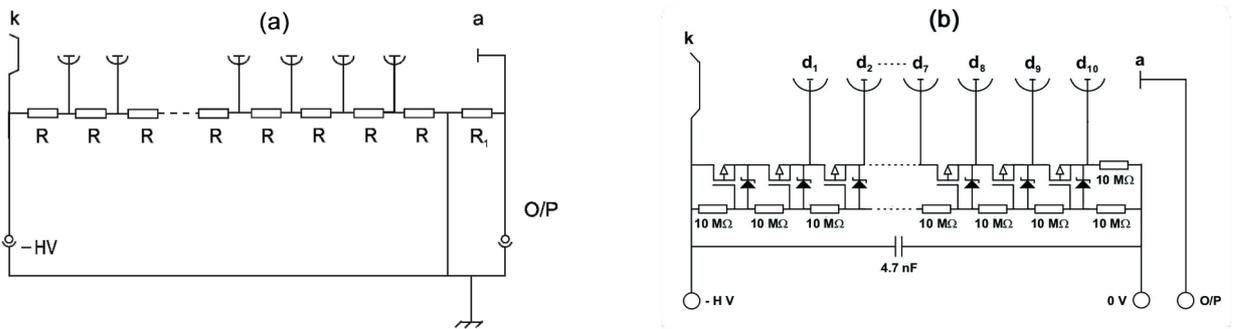
**figure 3** simplified voltage divider schematics (a) conventional type (b) the active divider in which the resistor and FET strings draw only  $\sim 5 \mu\text{A}$  each when  $I_a = 0$ . Otherwise the divider provides anode current,  $I_a$ , on demand with  $I_D = I_a + 10 \mu\text{A}$  where  $I_D$  is the current drawn from the supply.
