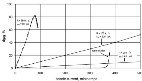
**figure 4** illustrating the superior performance of an active divider compared with conventional resistor types. One of the basic requirements of any detector is that its gain should remain constant and independent of input signal strength.
