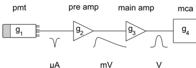
**figure 1** The overall sensitivity of a measuring system is proportional to the product of the gain of each element. This is illustrated for a scintillation counter where measurements are displayed on a multichannel analyser (mca). The skilled experimenter will always choose the optimal combination of  $g_1 \cdot g_2 \cdot g_3 \cdot g_4$  to achieve the required sensitivity.
