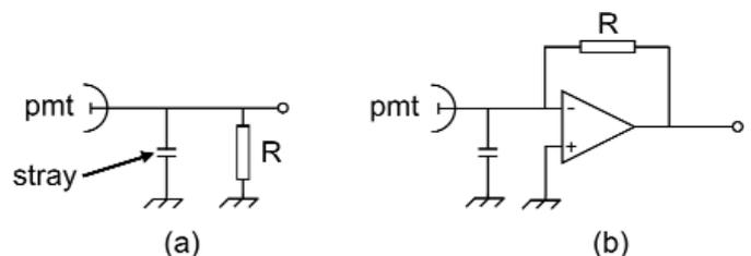
**figure 4 a)** Current to voltage conversion of the anode signal of a pmt. **b)** The transimpedance amplifier with its virtual earth input is ideally suited to a current generator, such as a pmt. The best amplifiers are still those made with discrete components although fast and stable op-amps are now more readily available. In practice R may be as high as 10 k $\Omega$  in (b) for fast applications
