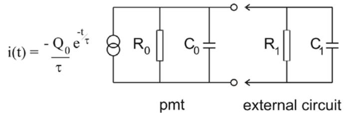
**figure 2** The equivalent circuit for a pmt is a current generator in parallel with  $R \gg 10^9 \Omega$  and  $C_0 \sim 5 \text{pF}$ . Most applications can be analysed in terms of an equivalent R and C combination. Without loss of generality we can take  $R_1 = R_0 R / (R_0 + R)$  and  $C = C_1 + C_0$ . In this example the current generator has been chosen to mimic a scintillator with decay time constant  $\tau$ .
