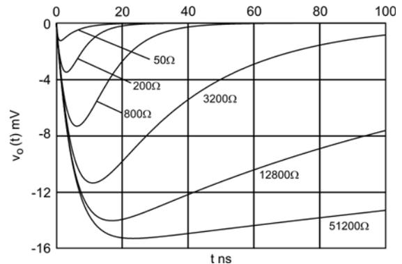
**figure 3** Evaluation of equation (2) for C = 10pF t = 5ns and g =  $10^6$  for various values of R. The amplitude and the shape of the pulses can be easily confirmed with a fast oscilloscope
