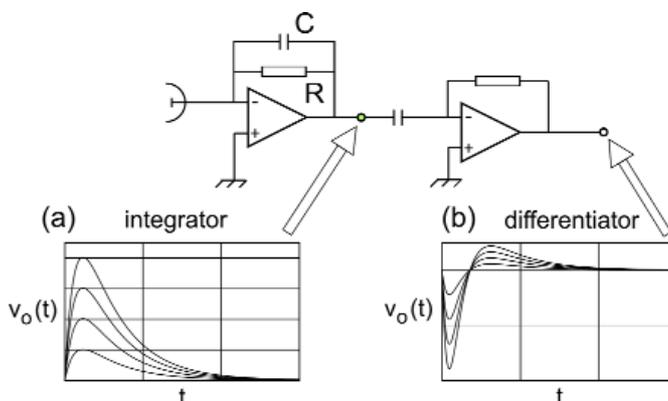
**figure 5** a) Capacitor C integrates the output from the pmt producing an output  $v(\text{max})$  of  $\sim Q/C$ . The reader can verify that a 1 MeV  $\gamma$  producing 6000 photoelectrons will generate a 1 volt output for  $C = 100 \text{ pF}$  with pmt gain =  $10^5$ . b) the “differentiating” amplifier produces bipolar pulses which cross the time axis at a common point. A zero-crossing discriminator detects the time of occurrence of this point.
