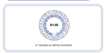
Our range of B14B sockets is available to suit the B14B hardpin base. The range includes versions with or without a mounting flange, and versions with contacts for mounting directly onto printed circuit boards.
