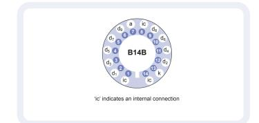
Our range of B14B sockets is available to suit the B14B hardpin base. The socket range includes versions with or without a mounting flange, and versions with contacts for mounting directly onto printed circuit boards.
