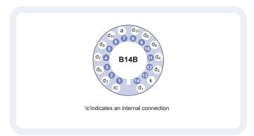
Our range of B14B sockets is available to suit the B14B hardpin base. The socket range includes versions with or without a mounting flange, and versions with contacts for mounting directly onto printed circuit boards.
