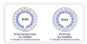
Our range of B19A sockets is available to suit the hardpin base. Our range of B14A sockets is available to suit the B14A cap. Both socket ranges include versions with or without a mounting flange, and versions with contacts for mounting directly onto printed circuit boards.
