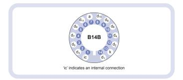
Our range of B14B sockets, available for this series, includes versions with or without a mounting flange, and versions with contacts for mounting directly onto printed circuit boards.
