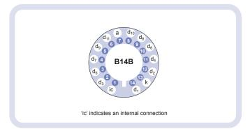
Our range of B14B sockets is available to suit the B14B hardpin base. The range includes versions with or without a mounting flange, and versions with contacts for mounting directly onto printed circuit boards.
