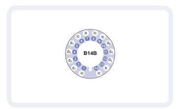
Our range of B14B sockets, available for this series, includes versions with or without a mounting flange, and versions with contacts for mounting directly onto printed circuit boards.
