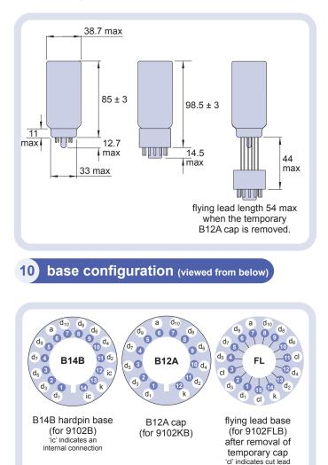
Our range of B14B sockets is available to suit the hardpin base. Our range of B12A sockets is available to suit the B12A cap. Both socket ranges include versions with or without a mounting flange, and versions with contacts for mounting directly onto printed circuit boards.
