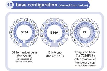
Our range of B14A sockets is available to suit the temporary B14A cap when the flying lead base variant is selected. The socket range include versions with or without a mounting flange, and with contacts for mounting directly onto printed circuit boards.
